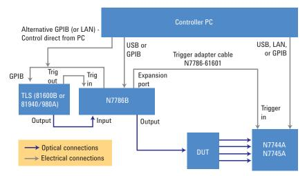
Figure 4. Schematic diagram of the instrument setup for single-sweep PDL measurement.
