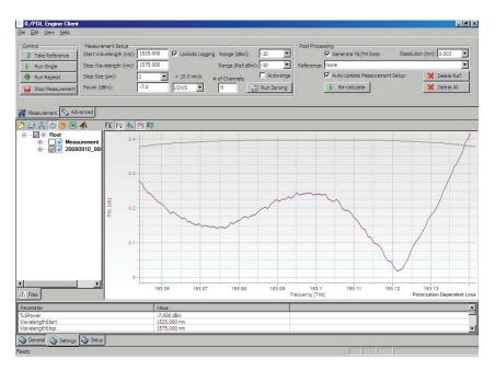
Figure 3. PDL measurement in the passband of a selected AWG channel.
