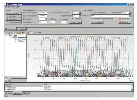
Figure 1. Example measurement of a 40 channel array waveguide multiplexer.
