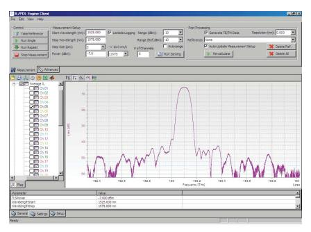
Figure 2. Insertion loss measurement for a selected AWG channel with about 60 dB measurement dynamic range.
