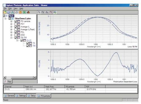
Figure 4. TE/TM analysis of a thin-film filter for the determination of PDf.
